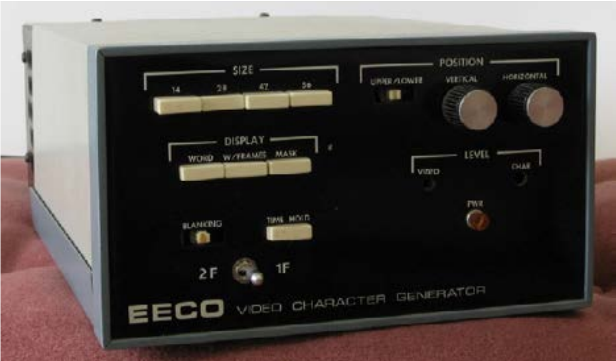
Fig. 2-2: EECO Video Character generator for burning timecode into analog video signals.
