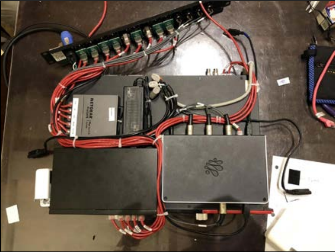
Fig. 4-24: Djesse tour second revision rack design - inner cabling routing
