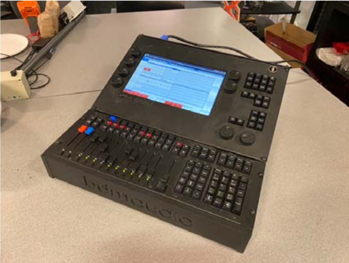
Fig. 5-4: Chamsys lighting desk used to develop gamma experiences. Custom hardware for lighting desk by Brian Mayton.
