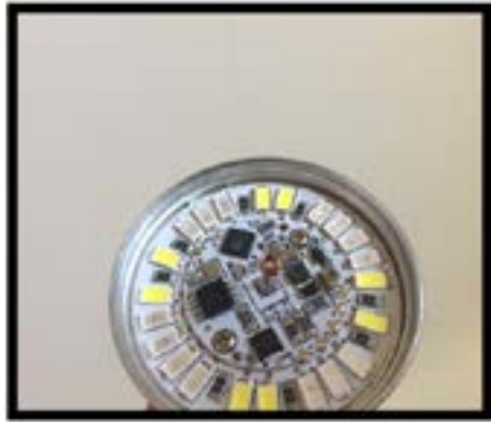
Fig. 5-2: ESP8266 based LED bulb - A19 form factor with custom firmware (Rieger , 2018)
