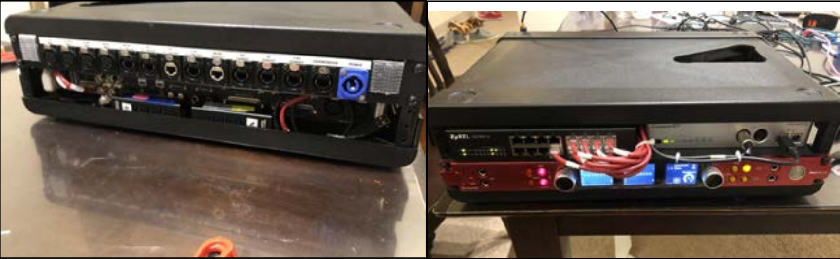
Fig. 4-25: Djesse tour second revision rack design - front and rear photos
