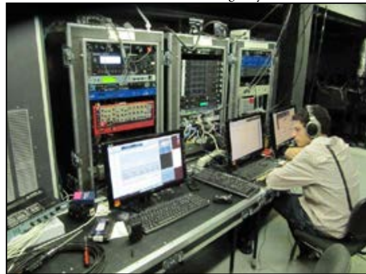
Fig. 3-8: The arrangement of computers and mixing desk for Death and the Powers . Computers from left to right: remote access to Synth, Effects, WFS, Ambisonics; WinControl and 3DAS, laptop with mixing notes and DCA Assignments, Studer Vista5 Control Console
